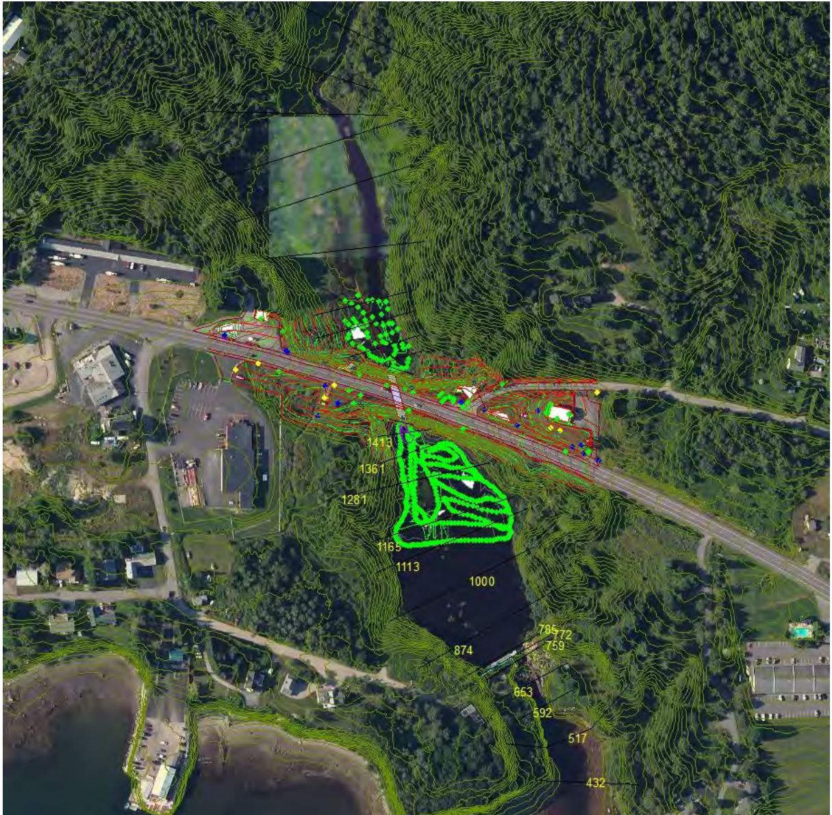
Figure 10. Survey (bright green and red) and LIDAR coverage (green contours) of project area. Geometric model cross sections are shown in black.
